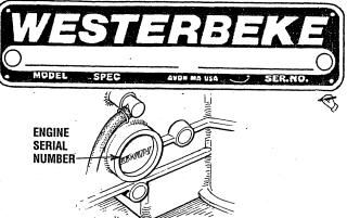
Take the time to enter this information on the illustration of the nameplate as shown above, as this will provide a quick reference when seeking technical information and/or ordering parts.
