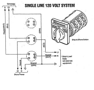
**CAUTION:** Damage to the generator can result if utility shore power and generator output are connected at the same time. This type of generator damage is not covered under the warranty; it is the installer's responsibility to make sure all AC connections are correct.
