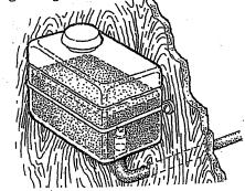
**NOTE:** This tank, with its short run of plastic hose, is best located at or above the level of the engine's manifold, but it can be located below the level of the engine's manifold if the particular installation makes this necessary.
