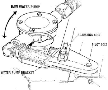
**NOTE:** The adjustment is the same for the FRESH WATER COOLED MODEL dual pumps.
