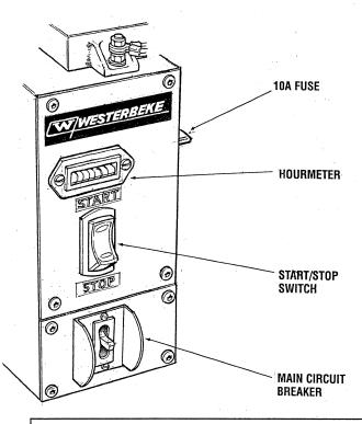
**WARNING:** Should the engine fail to start once the start switch has been depressed, a crank limit circuit will disengage the starter and stop the starting cycle. This will occur after approximately 15 seconds of cranking with no start.
