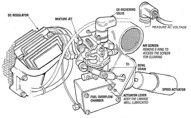
CARBURETOR WITH SPEED ACTUATOR
