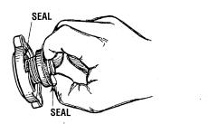
**NOTE:** Periodically check the condition of the pressure cap. Ensure that the upper and lower rubber seals are in good condition and check that the vacuum valve opens and closes tightly. Carry a spare cap.
